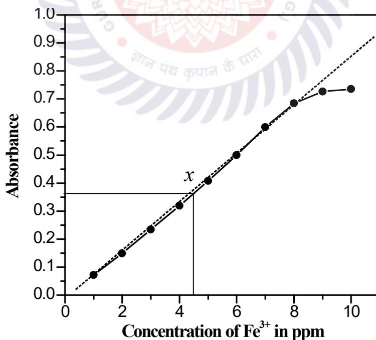
Fig. 1. Plot of absorbance versus concentration of Fe<sup>3+</sup> ion.
