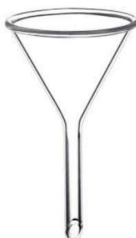
**FUNNEL :** Funnels are used for pouring liquids from one container to another. In addition, with the aid of filter paper, they can be used as separation devices to separate liquids from solids. It is fixed by a ring support on a stand.
