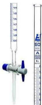
**BURETTE :** Burette is a vertical cylindrical piece of laboratory glassware with a volumetric graduation on its full length and a stopcock on the bottom. It is used to dispense known amounts of a liquid reagent in a titration experiment.
