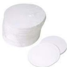
**Filter paper :** paper is used to separate solid particles from liquids. They can have different size with different pore size. Solids that remain on filter paper can later be dried on a watch glass or in an oven.
