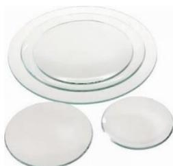
**WATCH GLASS :** Watch glass is used to allow crystal to dry after they have been filtered. They can be used as an evaporating surface or to cover a beaker that can be heated to very high temperatures.
