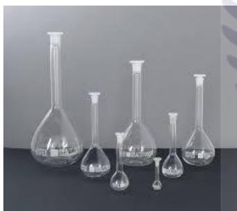
**VOLUMETRIC FLASK :** Volumetric flasks are used for measuring very precise and accurate amounts of aliquid and is used for such when the amount is too much for pipette or burette. They are also used for solution preparation.
