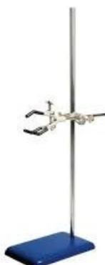
**STAND :** A metal rod attached to a heavy metal base. The heavy base keeps the stand stable, and the vertical metal rod allows for easy height adjustment of the iron ring/clamp.
