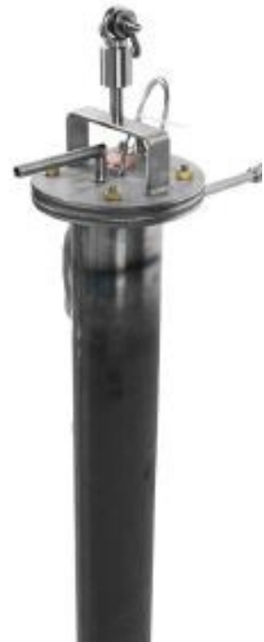
Fig. Coke reactivity test resort
